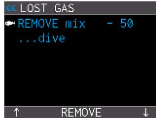
Mix 50% can be removed from the plan and the decompression calculations. It can be restored by repeating the same procedure.
