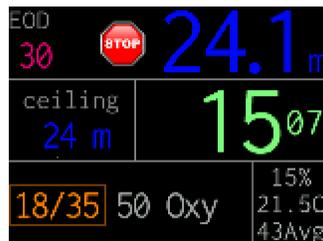
Direct ceiling display: deco ceiling limit with smiley depth guide.
